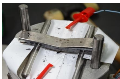
Fig. 8 Flexural test. Damping-metal deformed, and was not broken.
