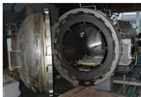
Fig.3 Autoclave (AC) apparatus used in this study
