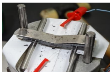
Fig. 8 Flexural test. Damping-metal deformed, and was not broken.
