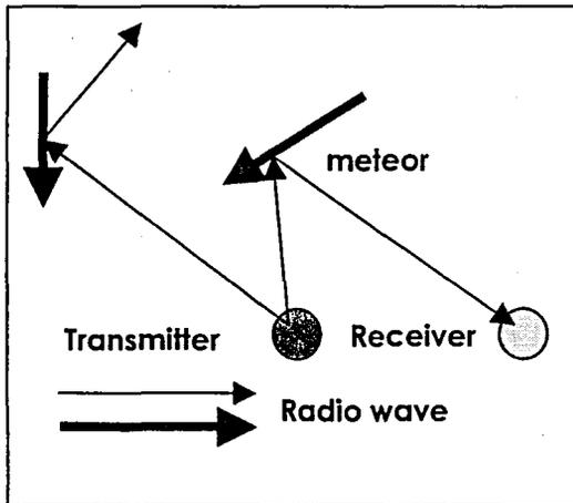
Fig.1 Radio reflection due to meter trails
