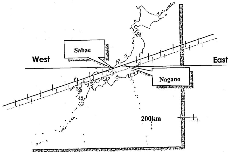
Fig.3 Baseline of the Transmitter and Receiver: Transmitter at Fukui National College of Technology (136.18E, 35.95N) in Sabae, Fukui, Japan Receiver at Nagano National College of Technology (138.18E, 36.63N) in Nagano, Nagano, Japan.
